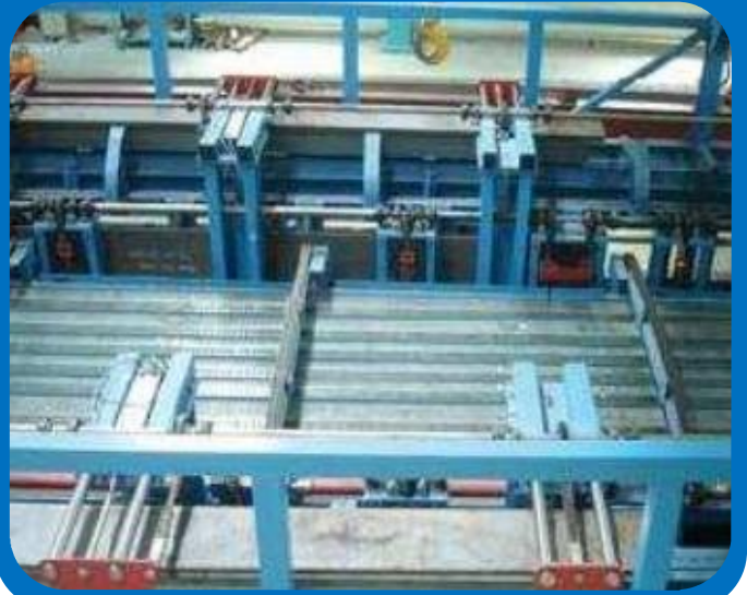
Flange cage &amp; conveyor
