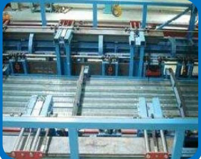
Flange cage & conveyor
