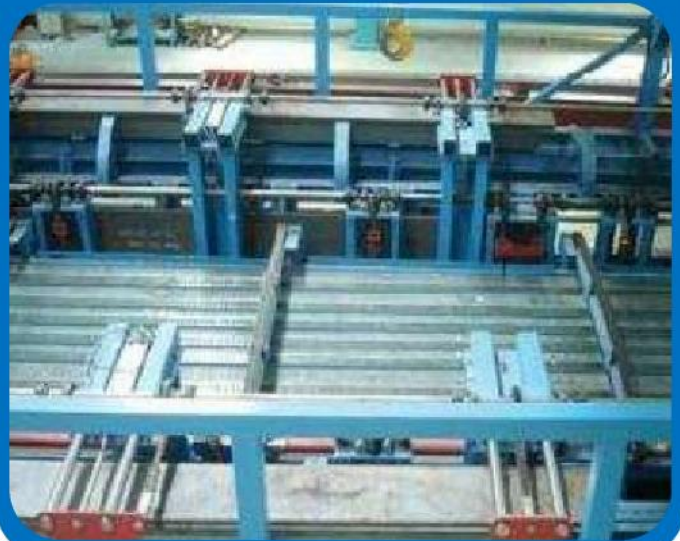
Flange cage & conveyor
