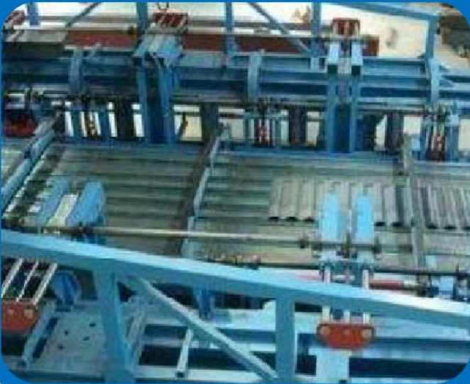
Corrugater web conveyor
